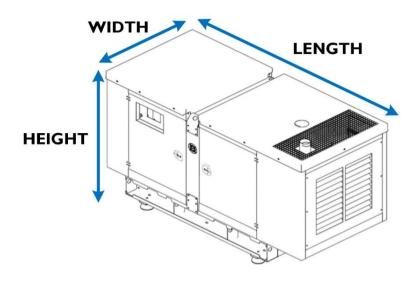
UJST (standard canopy dimensions are specified. Dimensions for UJBT (heavy-duty canopy) and UJPT (project type canopy) vary.
